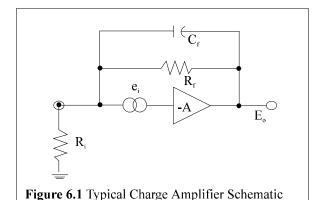
The feedback capacitor  $C_{\rm f}$  comes into play only in the dynamic situation and its influence does not affect the steady-state situation. The voltage  $e_{\rm i}$  is a DC offset voltage, usually very tiny (microvolts), that exists at the input gate of the MOSFET circuit. This minute leakage current exists in all real devices. As demonstrated in Equation 1, the steady-state (DC) output voltage  $E_{\rm o}$  is:
