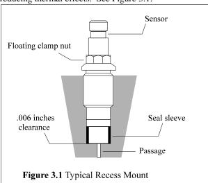
When using a recess mount, note that the length of the passage may limit the frequency range of the measurement. The effect the passage has is similar to that of an under-damped second order system, with the resonant frequency determined by passage length. The passage length thus limits pressure pulse rise time and may also cause passage ringing.
