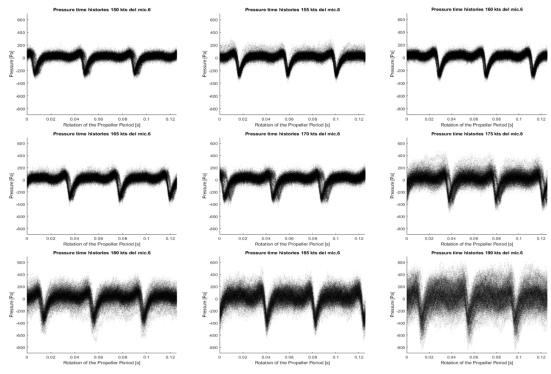
Figure 7 Pressure time history refer to propeller rotation period, mic. 6
