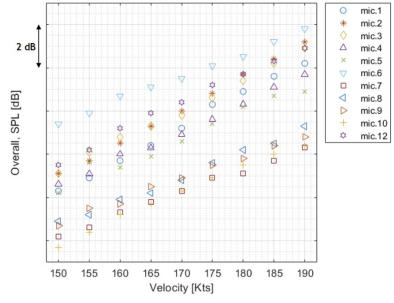
Figure 4 OASPL at different flight conditions
