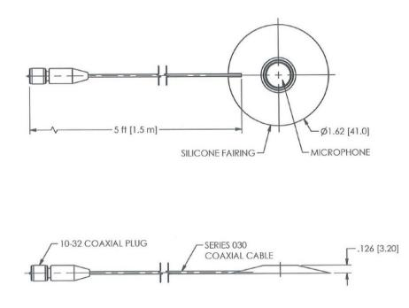
Figure 1 Surface microphone size
